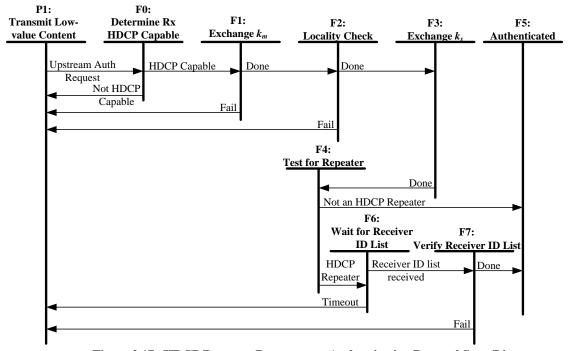
Figure 2.17. HDCP Repeater Downstream Authentication Protocol State Diagram
