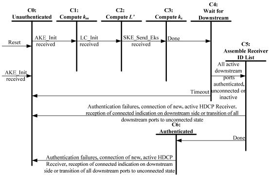
Figure 2.18. HDCP Repeater Upstream Authentication Protocol State Diagram
