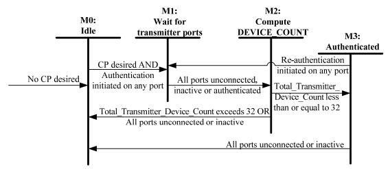
Figure 2.13. Main HDCP Transmitter Function State Diagram
