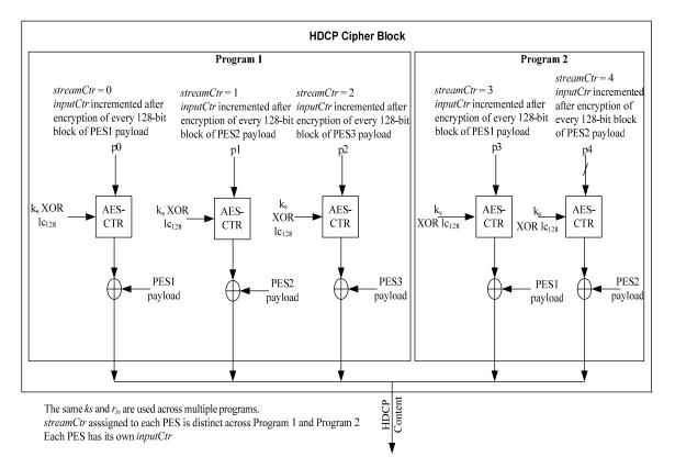
Figure 3.3. HDCP Encryption of Multiple Programs
