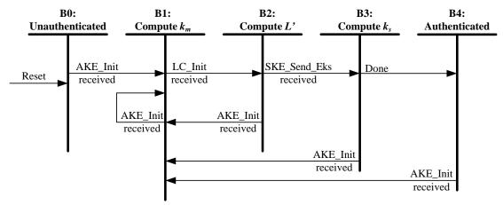
Figure 2.14. HDCP Receiver Authentication Protocol State Diagram
