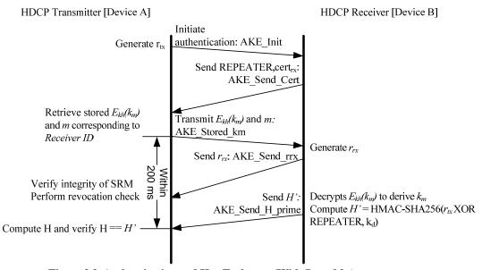
Figure 2.2. Authentication and Key Exchange (With Stored  $k_m$ )
