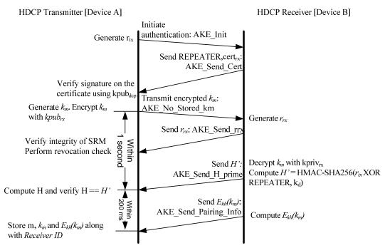
Figure 2.1. Authentication and Key Exchange (Without Stored  $k_m$ )
