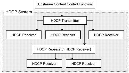
Figure 1.1. Sample Connection Topology of an HDCP System
