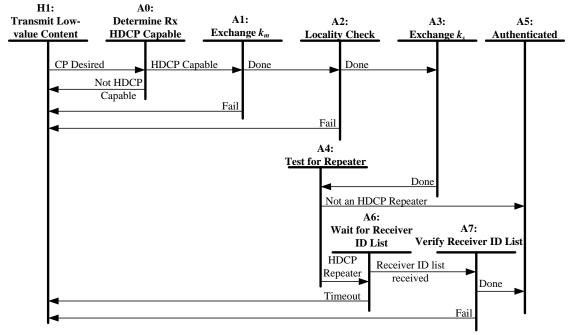
Figure 2.12. HDCP Transmitter Authentication Protocol State Diagram
