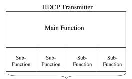
Sub-function on each port implements the HDCP Transmitter State Diagram
