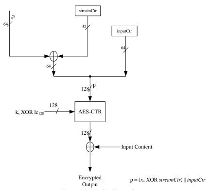
Figure 3.2. HDCP Cipher Structure
