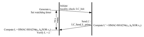
Figure 2.4. Locality Check between HDCP Transmitter and HDCP Receiver
