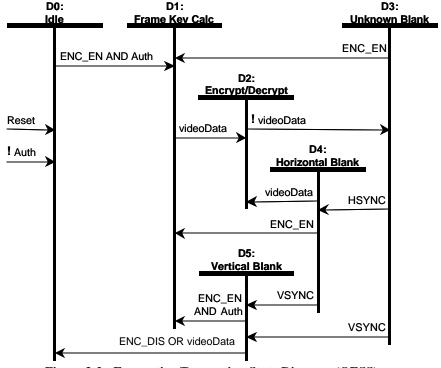
Figure 3-2. Encryption/Decryption State Diagram (OESS)
