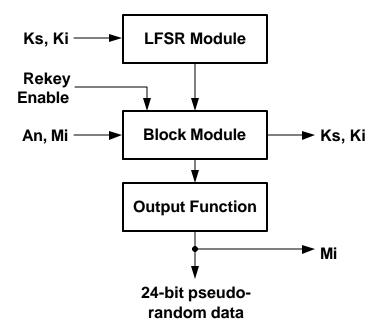
Figure 4-1. HDCP Cipher Structure
