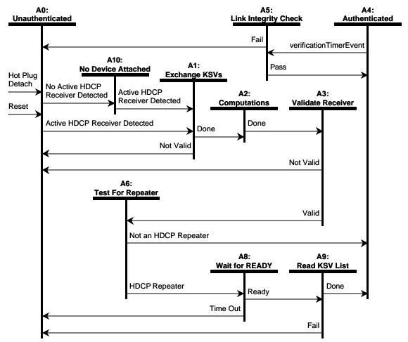
Figure 2-4. HDCP Transmitter Authentication Protocol State Diagram
