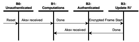
Figure 2-5. HDCP Receiver Authentication State Diagram
