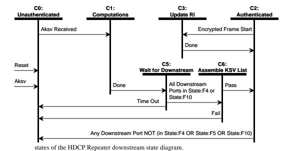
Figure 2-7. HDCP Repeater Upstream Authentication Protocol State Diagram
