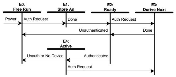
Figure 4-6. hdcpRngCipher State Diagram
