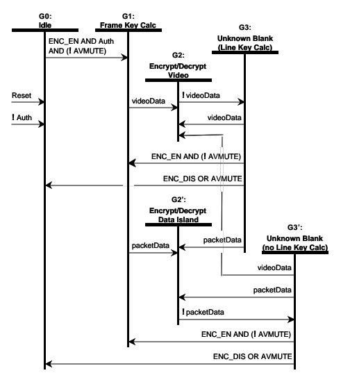
Figure 3-3. Encryption/Decryption State Diagram (EESS)
