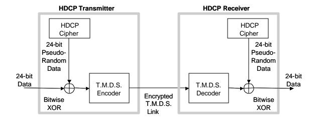
Figure 3-1. HDCP Encryption and Decryption
