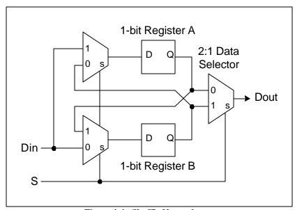
Figure 4-4. Shuffle Network
