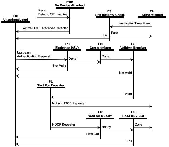
Figure 2-6. HDCP Repeater Downstream Authentication Protocol State Diagram
