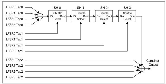
Figure 4-3. LFSR Module Combiner Function
